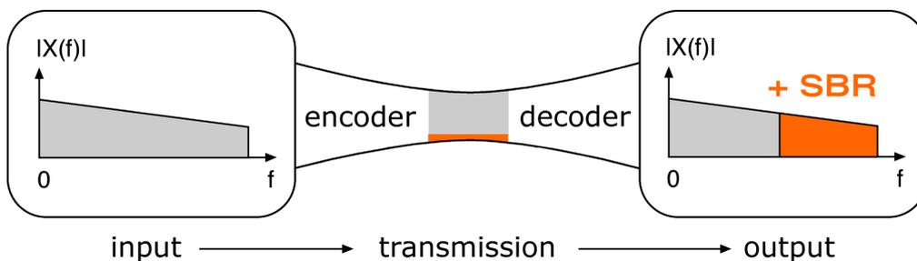
SBR can also improve the performance of narrow-band speech codecs, offering the broadcaster speech-only channels with 12 kHz audio bandwidth used for example in multilingual broadcasting. As most speech codecs are
